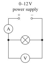
The student increased the output from the power supply from 0 V to 12 V in steps of 2 V. She recorded corresponding currents from the ammeter.
