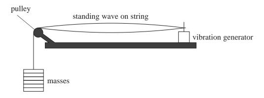
The standing wave had one antinode, as shown above, when the vibration generator had a frequency f.
